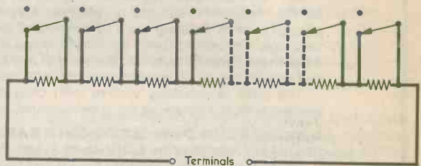
Fig. 2. An alternative approach towards making up a switched resistance box. There can be any number of switches and resistors
